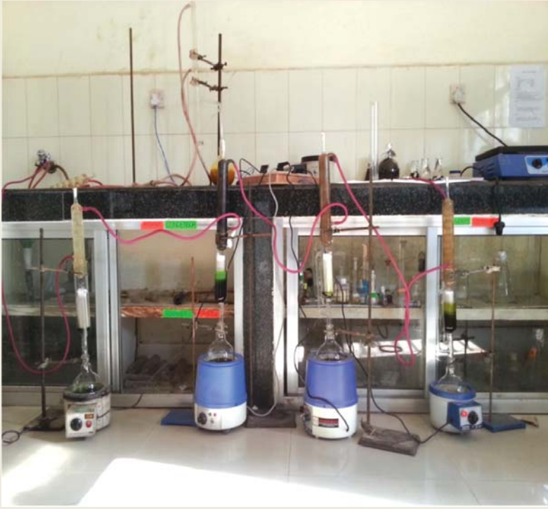
Soxhlet Extraction and Solvent - Solvent Extraction Method
